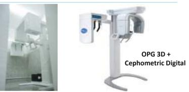
A Cephalometric radiograph is a radiograph of the head taken in a Cephalometer (Cephalostat)that is a head-holding device.
